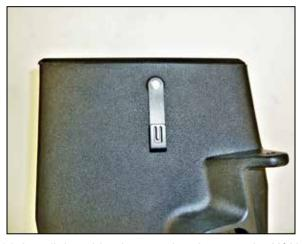
14. Install the wiring harness bracket onto the K&N air filter housing using the provided hardware.
