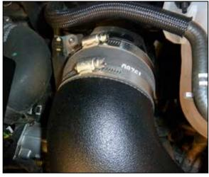
24. Secure the intake tube with the provided hose clamp.
