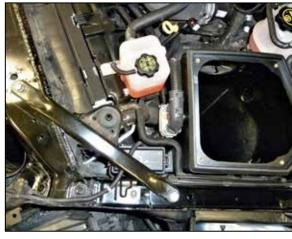
18. Reinstall the strut brace using the factory hardware. Resecure the relay box and expansion tank with the factory hardware.
