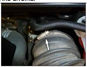
5. Loosen the hose clamp that secures the intake hose to the turbo inlet and disconnect the hose from the inlet.
