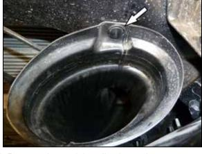
4. Remove the retaining clip shown that secures the fresh air duct and then disconnect the duct from the air filter housing.
