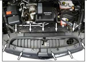
3. Remove the ten retaining clips that secure the valence and then remove the valence from the vehicle.
