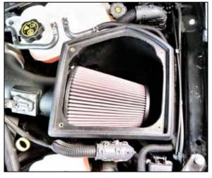
26. Install the K&N air filter into the air filter housing and onto the filter adapter, then secure with the provided hose clamp.
