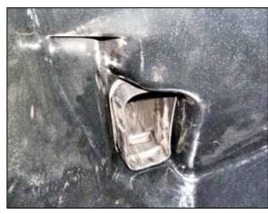
17. Engage the fresh air duct into the K&N air filter housing and then secure it with the factory retaining clip.
