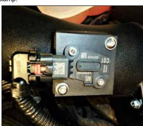
25. Reconnect the mass air sensor electrical connection.
