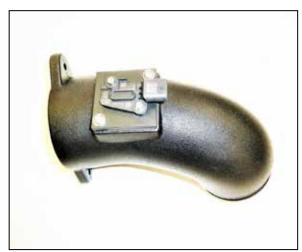
22. Install the mass air sensor into the K&N intake tube and secure with the provided hardware. Note the direction of the mass air sensor when installed should be as in the photo.
