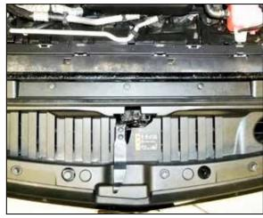
19. Reinstall the valence and secure with the factory retaining clips. Reinstall the hood release arm to the hood latch and secure with the factory bolts.
